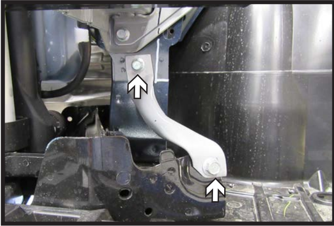
12. Using a 14MM socket, remove the two (2) bolts, and remove the brace.
