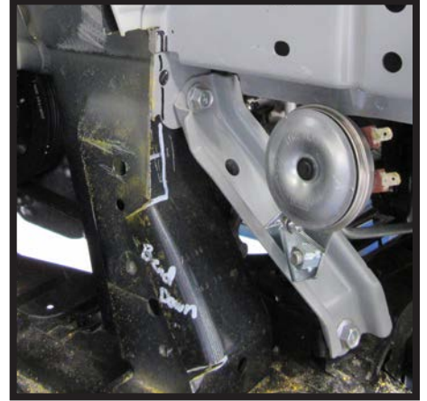
14. On the passenger side, measure down from the top of the frame extension 3" and mark. Mark out a notch from the 3" mark down to the bend flush with the inner frame side. Further down, make a mark at the bottom of the bend as deep as the upper notch (gray). Using a reciprocating saw, cut the bottom line (gray) and the bottom side of the upper notch. Bend the lip back towards the frame. Continue cutting out the upper notch flush to the inner frame. Treat the driver side similarly, starting just below the lower bolt. A completed picture of the passenger side is pictured.
