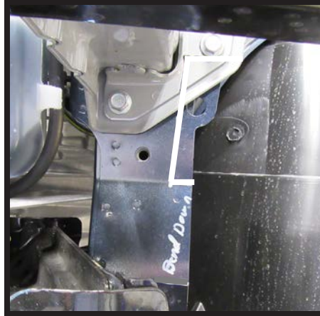
14. On the passenger side, measure down from the top of the frame extension 3" and mark. Mark out a notch from the 3" mark down to the bend flush with the inner frame side. Further down, make a mark at the bottom of the bend as deep as the upper notch (gray). Using a reciprocating saw, cut the bottom line (gray) and the bottom side of the upper notch. Bend the lip back towards the frame. Continue cutting out the upper notch flush to the inner frame. Treat the driver side similarly, starting just below the lower bolt. A completed picture of the passenger side is pictured.
