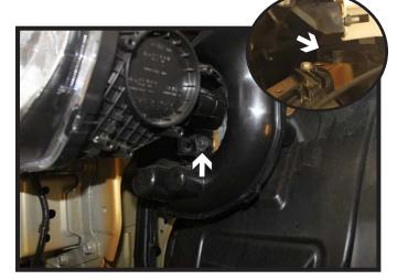
On the driver side, using a 10MM socket, remove the screw from the lower section of the baffle. Remove the push pin from the upper section just below the blinker (inset). Set the baffle aside.
