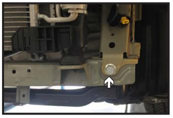
11. Using a 17MM socket, remove the two (2) bolts from the lower frame. There is one (1) on each side.
