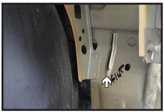
12. Using a hammer, flatten the ridge behind the frame webbing. Do this on both sides of the vehicle.
