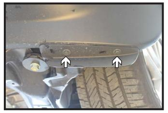
4. Using a 10MM socket, remove the four (4) screws from the underside of the fascia in front of the tire. There are two (2) on each side.
