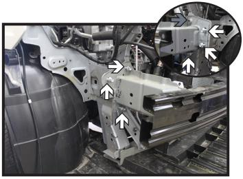
13. Using a 14MM socket, remove the three (3) bolts from the passenger side of the bumper. Then remove the three (3) bolts from the driver side (inset). Also remove the nut on the driver side with a 16MM socket (gray). Set the bumper aside.
