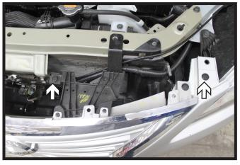
2. Remove the four (4) push pins from the top edge of the fascia. There are two (2) on each side.
