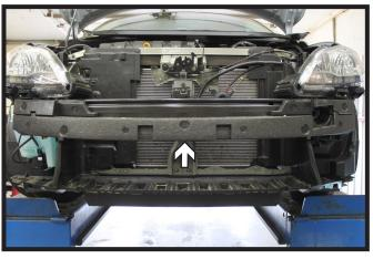
6. Pull the styrofoam support off the metal bumper.
