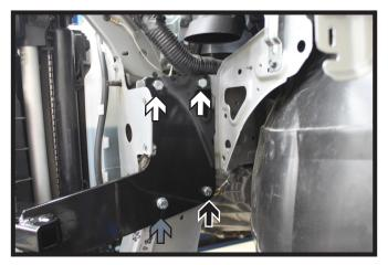
15. Using a 13/32" drill bit, drill the four (4) holes on the driver side and three (3) holes on the passenger side thru the frame. Install 3/8"-16 x 1-1/4" bolts with lock washers into all holes with 3/8"-16 hex nuts on the top four (4) holes of the baseplate (white) and 3/8"-16 nut plates on the front lower holes (gray). On the driver side lower back hole use three (3) 3/8" flat washer and a 3/8"-16 hex nut on the inside of the frame (black).
