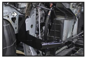
14. Flush the baseplate with the top of the frame, level and clamp into position.
