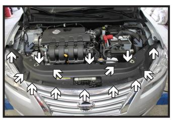
Using a 10MM socket, remove the two (2) bolts from the top edge of the fascia cover (gray). Then remove the fourteen (14) push pins from the cover (white). Set the cover aside.
