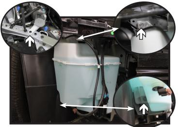
8. On the filler tube of the washer reservoir, remove the push pin by the filler cap (top left). Using a 10MM socket, remove the screws from the top (top right) and bottom (bottom right) of the reservoir. Disconnect electrical lines and plug fluid lines. Set the washer reservoir aside.
