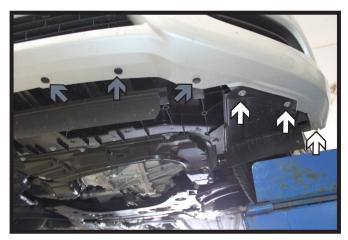
4. From the bottom edge of the fascia, using a 10MM socket, remove three (3) bolts (white). Then remove three (3) push pins (gray). Do this on both sides of the vehicle.
