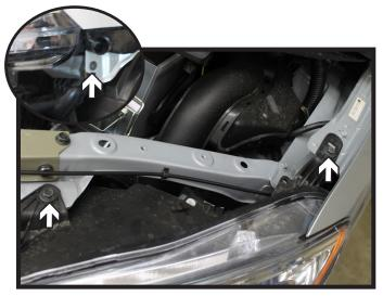
Using a 10MM socket, remove the two
