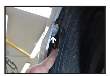
Using a 10MM socket, remove the bolt from behind the wheel well cover where the fascia meets the fender. Do this on both sides of the vehicle.
