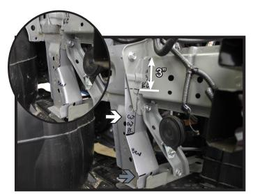
11. On the passenger side, measure down from the top of the frame extension 3" and mark. Mark out a notch from the 3" mark down to the bend flush with the inner frame side. Further down make a mark at the bottom of the bend as deep as the upper notch (gray). Using a reciprocating saw cut the bottom line (gray) and the bottom side of the upper notch. Bend the lip back towards the frame. Continue cutting out the upper notch flush to the inner frame.
