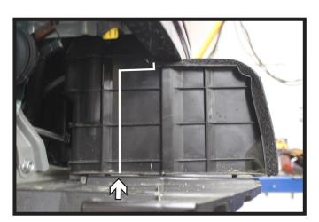
7. Trim the plastic shrouding approximately as shown for baseplate clearance. Do this on both sides of the vehicle.
