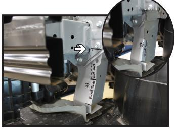
12. The driver side is cut similar to the passenger side only instead of measuring down 3" from the top of the frame extension, cut horizontally under the bolt head.
