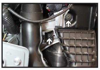
Using a 10MM socket, remove the three
