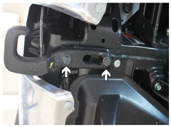
Using a 17MM socket, remove the two
