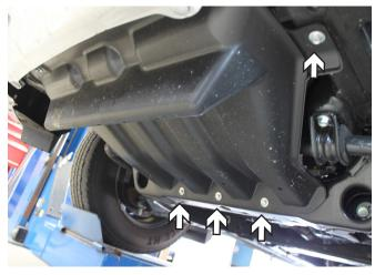
Using a 12MM socket, remove the three (3) rear bolts and the two (2) side bolts one on either side of vehicle from the belly pan.
