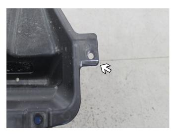
5. Trim the belly pan side tab as needed to clear baseplate on both sides of the vehicle. Reinstall belly pan using the existing bolts.
