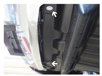
3. Using a 12MM socket, remove the front two (2) bolts from the belly pan and remove from the vehicle.
