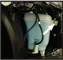
for the top, front hole. For this, use the 6MM-1.0 x 30MM hex head bolt and the 1/4" washer that has been provided.
