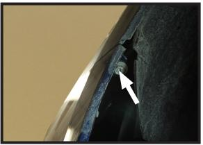
4. Pull the splash guard back slightly. At the top portion of the wheel well area is a 10MM bolt. Using a 10MM socket remove this bolt. Do this on **BOTH** sides of the vehicle.
