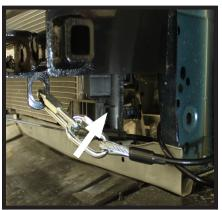
11. Attach the permanent baseplate safety cables to the provided convenience link on
