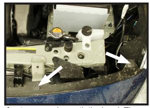
1. Remove the five (5) push pins that are located in the front area, underneath the hood. There are two (2) push pins located on the outer edges on **BOTH** the driver side and the passenger side. There is also one (1) located in the center.
