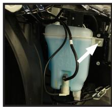
Reconnect the windshield wiper fluid reservoir using the existing fasteners except
