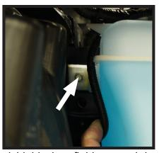
6. With a 10MM socket remove the three (3) bolts that hold the windshield wiper fluid reservoir in place. On the front of the reservoir there is one (1) bolt at the bottom and one (1) towards the top. On the backside of the reservoir is the 3rd bolt. It may be necessary to push back on the wheel well liner to access this bolt.
