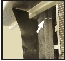
7. Release the push pin that is connected to the bumper. Using a utility knife cut straight across to remove the plastic guard. Do this on **BOTH** sides of the vehicle.
