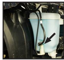
5. With a Phillips screwdriver, remove the screw on top of the windshield wiper fluid reservoir. Next, disconnect the tubes and plug to prevent leakage. Set the reservoir off to the side temporarily.
