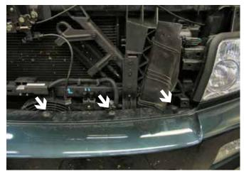
2. Remove 3 push pins from the front fascia on both sides of the vehicle. Just inside headlight assembly. (The driver's side of the vehicle is shown).
