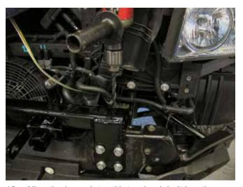
12. Align the baseplate with tow hook bolt locations. Finger tighten the 201-0153 hex bolts with lock washers. Slide 107-2681 between the top of the frame and back hole in baseplate. Tighten the 8-201-0153 hex bolts. Using the baseplate as a template, drill the back hole of the baseplate into the top of the frame with 17/32" drill bit, this will need to be done on both sides of the vehicle. Then install the last bolt.\*\*
