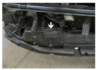
9. Remove push pin on top of where the tow hook attaches to the metal bumper. Take plastic cover off and set aside (please remember to return these to the customer as they are **NOT** reinstalled on the vehicle). This is done on both sides of the vehicle. (The passenger's side is shown).\*\*
