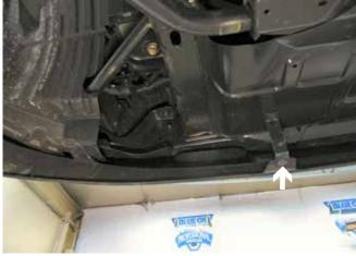
6. Remove 2 Phillips push pins from the underside of the front fascia below the belly pan. (The driver's side is shown.)
