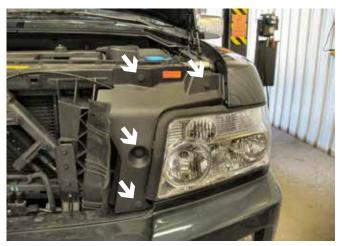
Remove 4 push pins from the front fascia near each headlight housing.
