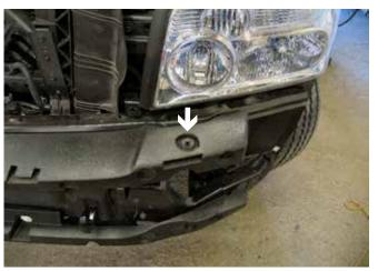
Remove the 3 push pins on top of the Styrofoam, pull forward and set the Styrofoam aside. (The driver's side is shown.)
