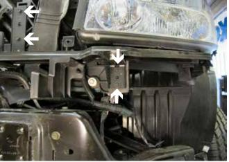
11. Remove 8 metric bolts with a 10MM Socket from the metal fascia support bracket, 4 metric bolts need to removed from the hood latch. Which located right behind the metal fascia support bracket. Remove bolts from both sides. Pull forward on the bracket to remove it and set it aside. (The driver's side is shown.)\*\*
