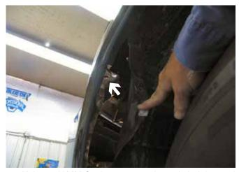
4. Using a 10MM Socket, remove 1 metric bolt located in the wheel well. Set this bolt aside. This is done on both sides. (The driver's side is shown).
