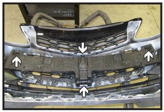
Remove the foam piece from the back side of the fascia by releasing the four (4) clips holding it in place. This will not be reinstalled later.
