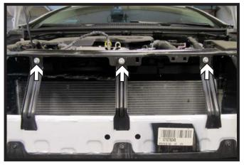
Using a 10MM socket, remove the three
