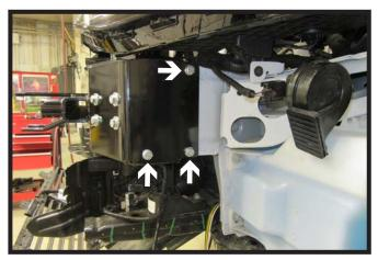
12. Using a 3/8" drill bit, drill out the three (3) holes for the side plate. Be careful not hit any wires while drilling. Then insert the three (3) 3/8" bolts with lock washer and 3/8" whiz nut with wire. Do this on both sides of the vehicle.
