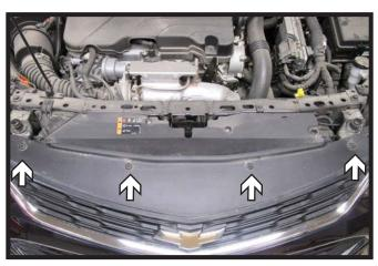
1. Using a 7MM socket, remove the four (4) bolts from the top of the fascia cover.
