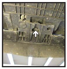
3. Using a 7MM socket, remove the ten (10) bolts from the underside of the vehicle. There are five (5) on each side of the car. Remove the one (1) push pin from the center of the underside.
