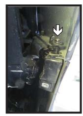
2. Using a T15 Torx, remove the two screws from the edge of the wheel well in front of the tire. Next, pull the cover back. Using a 7MM socket, remove the one (1) bolt from under the cover. Do this for both sides of the vehicle.
