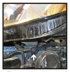
6. Using a 7MM socket, remove the five (5) bolts from the headlight. There are three (3) on top of the headlight area, and two (2) below the headlight on the side. Remove the headlight and set aside. Do this for both sides of the vehicle.
