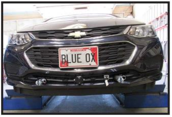
12. Hold the fascia as close to its original position, mark and trim the fascia around the convenience links and attachment tabs. Reinstall the center brace, headlights, fascia and fascia cover.
