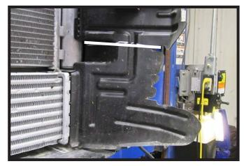
5. Using a reciprocating saw, trim the marked areas on the bumper plastic shielding.
