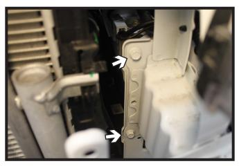
6. Using a 12MM socket, remove the two (2) bolts from the inside edge of the bumper. Do this on both sides of the vehicle.
