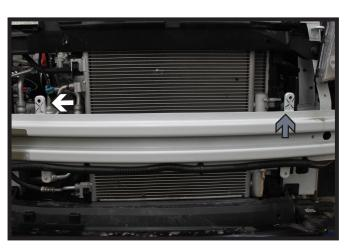
Bend the passenger side bumper tab back slightly for baseplate clearance (white).
