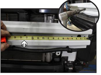
10. Using a 3/8" drill bit, drill a hole thru the bumper 13-1/2" in from the end. Repeat on the other side of the vehicle.
