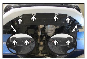
3. Using a phillips screwdriver or 7MM socket, remove the eight (8) screws from the bottom edge of the fascia. There are four (4) on each side of the vehicle.
