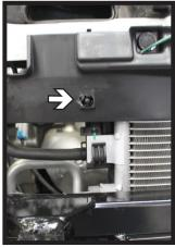
12. Trim the passenger side baffle around the baseplate and reinstall. Reinstall the temperature sensor into the baffle (right).
