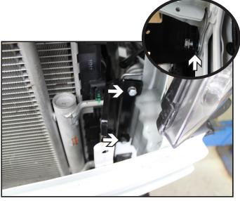
8. Install the driver side end plate onto the frame with 8MM-1.25 x 35MM bolts and 8MM lock washers. Use two (2) 1/4" flat washers per bolt as a spacer between the frame and the end plate. Do not fully tighten the bolts until the baseplate is installed. Repeat on the passenger side.
