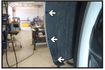
In the wheel well, using a T20 Torx, remove the three (3) screws from the outer edge. Do this on both sides of the vehicle.
