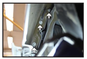
4. Behind the wheel well cover further back from the previous screw, using a 7MM socket, remove the three (3) screws from the fender. Do this on both sides of the vehicle.
