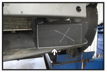
8. Trim the plastic shrouding on the underside of the bumper as shown for baseplate installation. Do this on both sides of the vehicle.
