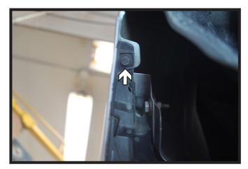
Behind the wheel well cover, using a 7MM socket, remove the screw from the fascia joint. Do this on both sides of the vehicle.
