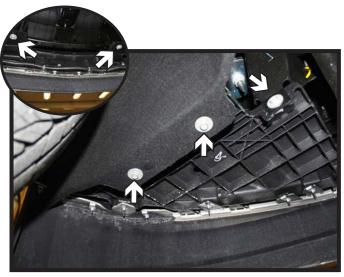
4. Using a 10MM socket, remove the eight (8) screws from the underside of the fascia. There are three (3) on each side and two (2) in the middle.
