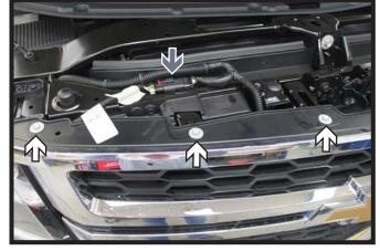
Using a 10MM socket, remove the six (6) screws from the top edge of the fascia (white). There are three (3) on each side. On the passenger side, disconnect the wiring harness (gray).
