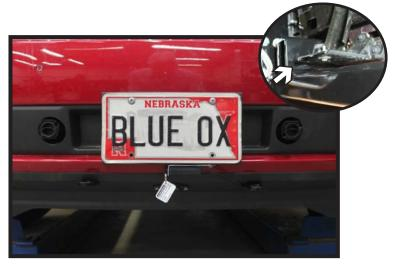
14. Reinstall the fascia and fascia cover. Note: The inside fascia brackets may need to be bent upwards slightly to reinstall the inner screws (inset).
