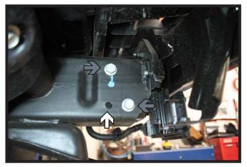
6. Using a 17/32" drill bit, drill out the existing hole in the bottom of the frame thru the ACC bracket (white).
