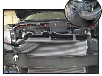
6. Using a 7MM socket, remove the screw from the front of the baffle (white). Then remove the rear push pin (inset) and the push pins on top towards the driver side (gray). Remove the baffle from the vehicle and set aside.
