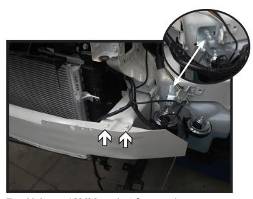
Using a 13MM socket & wrench, remove the four (4) bolts from the top edge of the bumper. There are two (2) on each side.
