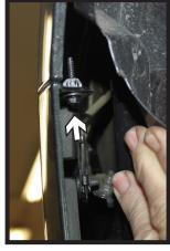
2. Using a T15 Torx, remove the three (3) screws from wheel well (left). Pull back the wheel well liner and remove the screw at the fascia joint with a 7MM socket (right). Do this on both sides of the vehicle.
