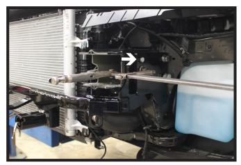
11. Position the baseplate onto the vehicle in between the frame and support plate. Line up the holes of the baseplate and support plate and securely clamp in place.
