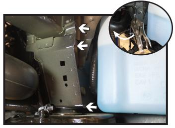
8. Using a reciprocating saw, cut the frame face back flush to the frame side rail in the three (3) areas indicated. Bend the frame face forward so it is flush to the frame side rail (inset). Do this on both sides of the vehicle.
