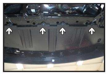
4. Remove the four (4) push pins from the underside of the fascia.
