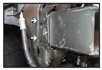
Using a 18MM socket, remove the two
