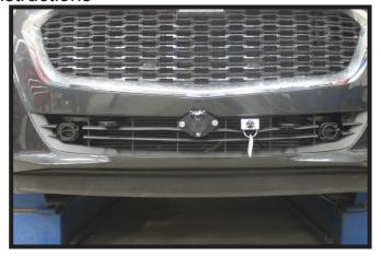
14. Hold the fascia as close to its original position, mark and trim the fascia around the convenience links and attachment tabs. Reinstall the air baffle, PS headlight, bumper, horn and fascia.
