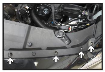
1. Using a T20 Torx, remove the eight (8) screws from the top edge of the fascia. There are four (4) on each side.
