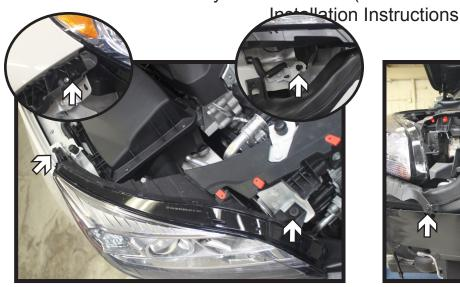
Using a 7MM socket, remove the four (4) screws from PS headlight. There are two (2) on the top side, one (1) along the side (left inset) and one (1) underneath (right inset). Disconnect the electrical line and set the headlight aside.
