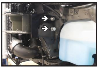
10. Install the support plate onto the vehicle with 12MM-1.75 x 50MM bolts with 12MM lock and flat washers. Level the plate and temporarily snug the bolts. Do this on both sides of the vehicle.
