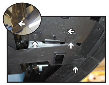
Using a 7MM socket, remove the ten (10) screws from the underside of the fascia. There are five (5) on each side.
