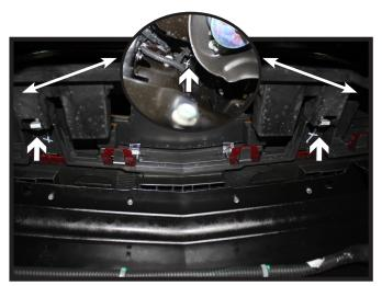
Using a 10MM socket, remove the four (4) screws from the underside of the fascia. There are two (2) in the middle and one (1) on each side.
