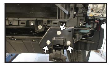
Using a 15MM socket, remove the three (3) bolts from the cover plate. Do this on both sides of the vehicle.
