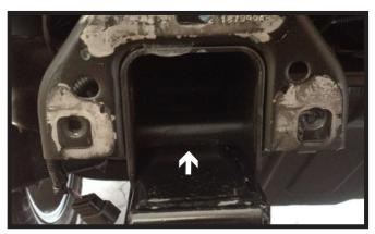
8. Using a 18MM socket/wrench, remove the two (2) bolts from the tow hook. Do this on both sides of the vehicle (left).
