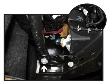
Using a 15MM socket, remove the bolt from the bumper reinforcement bar. Do this on both sides of the vehicle. Disconnect the running lights/electrical connections (gray) and set the bumper aside.
