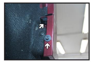
Using a 7MM socket, remove the two (2) screws from the wheel well. Do this on both sides of the vehicle. Unsnap the fascia from the body and set aside.
