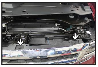
Using a 10MM socket, remove the four (4) screws from the top edge of the fascia. There are two (2) on each side.
