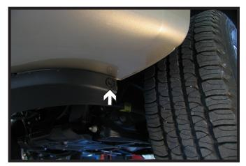
4. Remove the push pin from the underside of the fascia in front of the tire. Do this to both sides of the vehicle.
