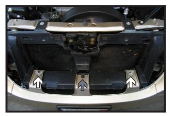
3. Using a 10MM socket, remove the two (2) screws from the top edge of the fascia (white). Then remove the push pin (gray).
