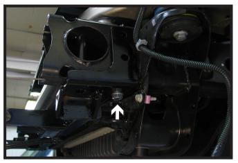
12. Using a 17/32" drill bit, drill the underside baseplate hole thru the frame. Install a 1/2"-13 x 1-3/4" bolt and a 1/2" lock washer into the hole with a 1/2" nut plate on the inside of the frame. Fully tighten the hardware. Do this on both sides of the vehicle.
