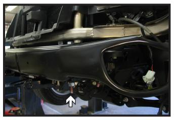
14. Reinstall the bumper using the supplied 5/8"-11 x 8" bolts, 5/8" flat & lock washers and 5/8"-11 hex nuts.
