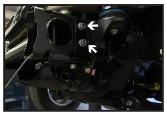
13. Using a 17/32" drill bit, drill the two (2) side baseplate holes thru the frame. Install a 1/2"-13 x 1-3/4" bolts and a 1/2" lock washers into the holes with a 1/2" nut plates on the inside of the frame. Fully tighten the hardware. Do this on both sides of the vehicle.
