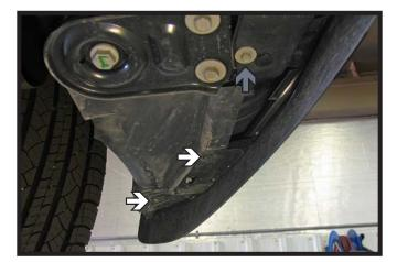
5. Remove two (2) Phillips screws from under the fascia with a screwdriver. Using a 10MM socket, also remove the hex bolt from under the fascia (gray arrow). Do this to both sides. Pull fascia corners to the side of vehicle to release, then pull fascia forward and set fascia aside carefully for later reinstallation along with bolts.
