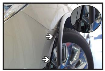
On 2012 models only: Once the previous step has been completed, gently pull the wheel well liner back and unclip the two (2) clips to loosen the outer trim.
