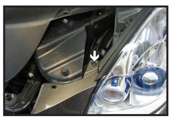
2. Using a Phillips screwdriver, remove a screw connecting the fascia near the headlight. Do this to both sides and set aside bolts for reinstallation later.
