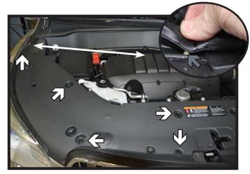
1. Remove the five (5) push pins from the top fascia cover (white). Then pry up the end of the rubber strip, releasing the clip underneath (gray). Do this on both sides of the vehicle. Remove the cover from the vehicle.
