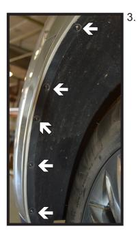
Using a T20 Torx, remove the five (5) screws from the outer edge of the wheel well.
