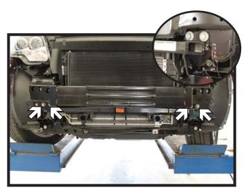
Using a 15MM socket, remove the four
