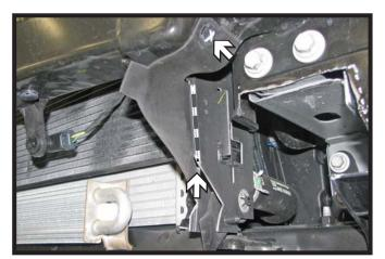
3. On the driver side, remove the push pin from the top of the plastic air deflector and trim as shown.
