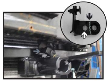
Hold the temperature sensor back to its original position and mark for trimming (black). Using a 7/16" drill bit, drill a new hole into the bracket on the other side of the trim line (white). Trim off the excess bracket, reinstall to the vehicle and reinstall the sensor to the bracket (gray).
