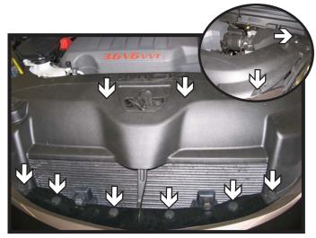
Remove twelve (12) push pins from the plastic piece covering the top of the under carriage with a flat screwdriver. There are two (2) push pins on each outer edge of the vehicle (see insert). Also, remove six (6) additional push pins from the bottom segment of the fascia. Remove push pins and set aside for later reinstallation.
