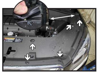
1. Remove the five (5) push pins from the top fascia cover (white). Then pry up the end of the rubber strip, releasing the clip underneath (gray). Do this on both sides of the vehicle. Remove the cover from the vehicle.
