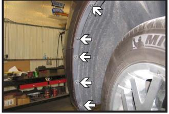
3. Remove five (5) Phillips screws just forward of the front tire, on the edge of fascia with a Phillips screwdriver. Do this to both sides of the vehicle. Set push pins aside to be reinstalled later.
