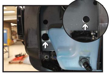
Using a 1-1/4" hole saw, drill an access hole into the frame for nut plate installation. Do this on both sides of the vehicle.
