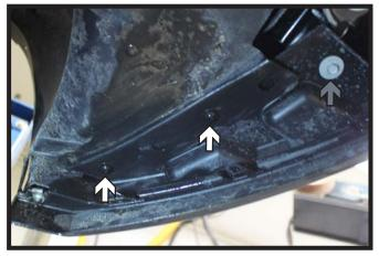
On the underside corner of the fascia, using a T20 Torx, remove the two (2) outer screws (white). Then using a 10MM socket, remove the one (1) inner screw (gray). Do this on both sides of the vehicle. Remove the fascia from the vehicle and set aside.
