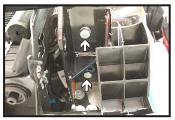
Using a 17/32" drill bit, drill the two (2) holes on the underside of the baseplate. Install 1/2"-13 x 1-1/2" bolts with 1/2" lock washers into the holes with 1/2"-13 nut plates inserted from the access hole. Do this on both sides of the vehicle.
