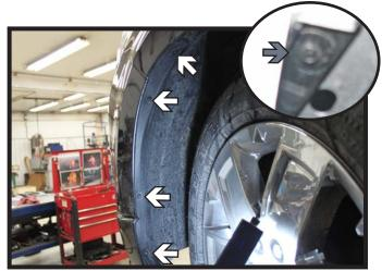
3. Using a T20 Torx, remove the four (4) screws from the outer edge of the wheel well (white). Then behind the wheel well cover, using a 7MM socket, remove the outer screw (gray). Do this on both sides of the vehicle.
