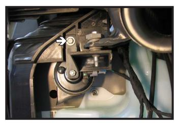
Using a 10MM socket, remove the hex bolt holding the horn to the frame rail. Remove the horn and bolt and set aside for later reinstallation. Do this to both sides.
