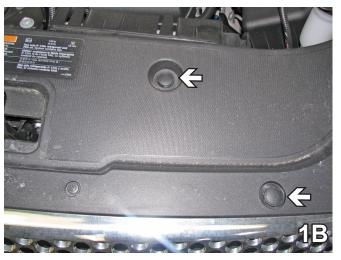
1. Using a flat screwdriver, remove three push pins from the flat plastic cover on top. Do this to both sides of the vehicle. Set push pins and top cover aside to be reinstalled later.
