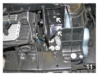
11. Using the baseplate as a template, drill the two (2) bottom holes into the frame with a 17/32" drill bit. Insert the 1/2"-13 nut plates into the frame (step 10) and align with drilled holes. Insert 1/2"-13 x 1-1/2" hex bolts and 1/2" lock washers into each hole and tighten down. Be sure to use Loctite Red on all bolts. Do this to both sides of the baseplate.
