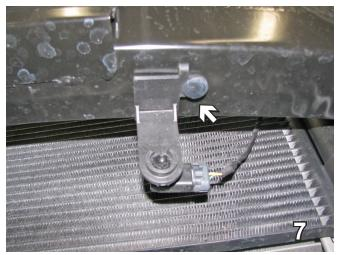
7. Remove the push pin holding the temperature sensor bracket below the bumper on the driver side. Unplug and set aside to be reinstalled later.
