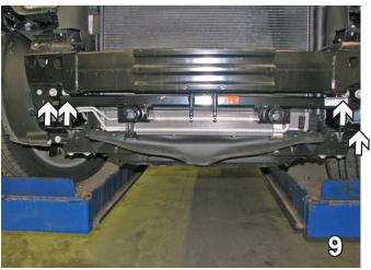
9. Using a 15MM socket, remove two (2) bolts from the front of the bumper. Do this to both sides of the bumper. Slide baseplate straight back, so that the holes on the baseplate line up with the existing holes of the bumper. Reinsert the existing bolts and tighten down, so the bolts are snug. Be sure to use Loctite Red on all bolts. Do this to both sides of the baseplate.
