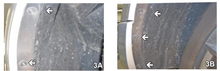
3. Using a T20 Torx, remove five (5) screws just forward of the front tire, on the wheel well. Do this to both sides of the vehicle. Set screws aside to be reinstalled later.
