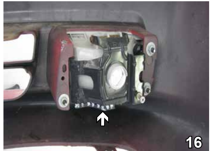
16. On the back side of the fascia, cut the 1/4" lower lip off of the running lights. Then cut 1" off 1/2" down from the bend, both sides.
