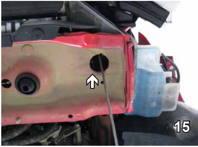
15. Using the 1 1/2" hole saw, cut a hole into the bottom of frame extension just below tie down bracket, both sides.
