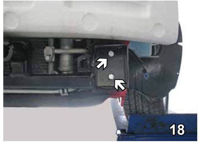
18. Using the baseplate as a template, drill the two holes on the front of baseplate with the 13/32" drill bit. Insert the 3/8-16 nut plates into the 1 1/2" drilled hole in lower frame extension to tighten with 3/8-16 x 1 1/4" bolts and 3/8" lock washers, both sides. Use loctite on bolts.
