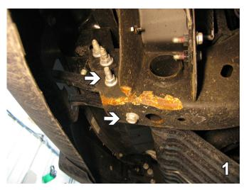
Using the 18MM socket, go up in behind to remove the bottom two metric bolts from the tow hook. Do this to both sides of the vehicle. Pull the tow hook forward and set aside. The tow hooks will not be reinstalled.
