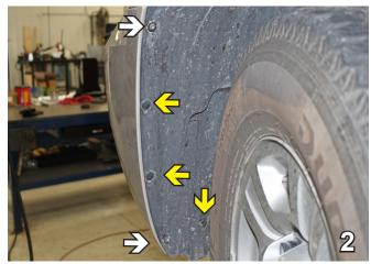
In front of the tire, remove two bolts with a 7MM socket (white arrows). Using a flat screwdrive, remove three push pins (yellow arrows). Do this to both sides of the vehicle. Set bolts and push pins aside to be reinstalled later.
