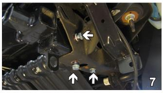
7. Slide baseplate in where the tow hooks were removed. Insert a 1/2-13 x1 1/4" hex bolt with loctite and 1/2" lock washer into the two holes on the side and the two holes on the bottom of the baseplate and tighten bottom two down first. Do this to both sides of the
