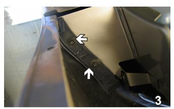
Using a 10MM socket, remove two bolts located just behind the wheel well plastic that we removed the bolts and push pins from. Do this to both sides of the vehicle. Set bolts aside to be reinstalled later.
