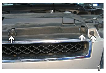
Remove three bolts with a 10MM socket. Do this to both sides of the vehicle. Set bolts aside to be reinstalled later.
