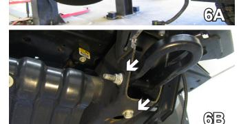
Using a 18MM socket, remove one bolt from the side and one bolt from the bottom of the tow hook. Do this to both sides of the vehicle. Factory tow hooks and bolts will not be reinstalled.
