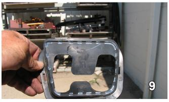
Using a utility knife, trim following the ridge around the backside of the guard where the tow hooks were. The photo above is what the opening should look like after your finished. Do this to both sides of the vehicle.
