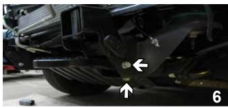
Using a 18MM socket, remove one bolt from the side and one bolt from the bottom of the tow hook. Do this to both sides of the vehicle. Factory tow hooks and bolts will not be reinstalled.
