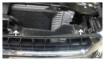
Once top plastic piece is set aside, you will need to remove two bolts with a 10MM socket. Do this to both sides of the vehicle. Set bolts aside to be reinstalled later.
