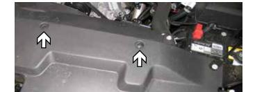
Using a flat screwdriver, remove four push pins from the flat plastic piece on top. Do this to both sides of the vehicle. Set push pins aside to be reinstalled later.
