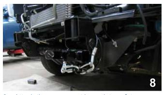
Attach the permanent baseplate safety cables to the provided convenience link on the baseplate. The photo above shows the recommended installation of the cables to frame of vehicle. Additional options may BE SURE TO USE LOCTITE® RED ON ALL BOLTS
