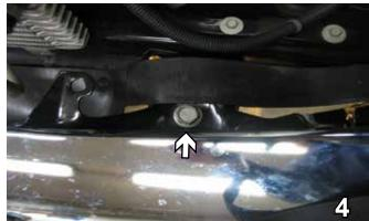
Using a 18MM socket, remove one bolt located just behind metal bumper, on top of bumper bracket. Do this to both sides of the vehicle. Set bolts aside to be reinstalled later.
