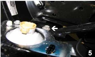
Using a 15MM socket, remove one bolt located underneath right in front of the tire.
