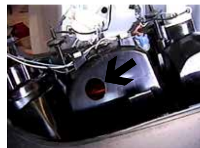
Location for the BX8869, top view of driver's side tail light assembly.
