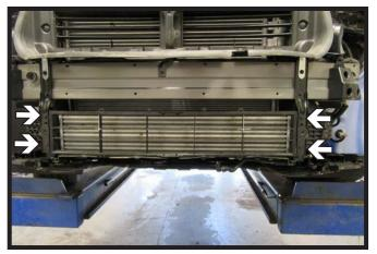
Using a 25 Torx socket, remove the four (4) screws from the lower grille and set it aside. It will not be reinstalled.
