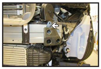
9. Remove the push pin from plastic reinforcement on the bumper face and set aside. Do this on both sides of the vehicle.
