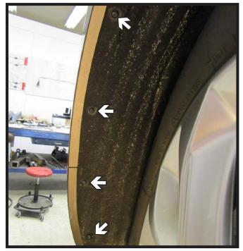
Using a T15 Torx socket, remove the four (4) screws from the wheel well liner. Do this on both sides of the vehicle.
