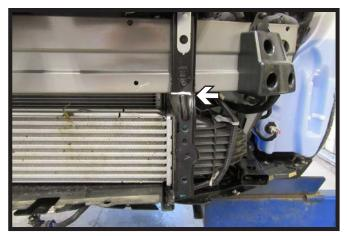
Using a reciprocating saw, trim the bracket flush with the bottom side of the bumper. Do this on both sides of the vehicle.
