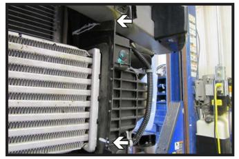
8. Trim the plastic shielding off flush under the bumper and across the bottom as shown. Do this on both sides of the vehicle,
