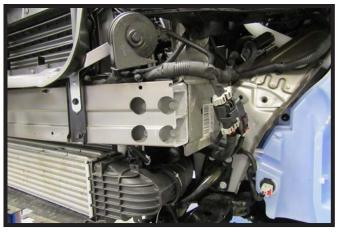
10. Using a reciprocating saw, trim the end of the bumper flush with the outside of the frame. Do this on both sides of the vehicle.
