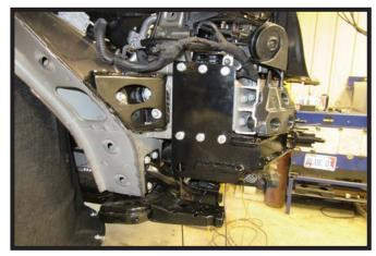
11. Flush the baseplate with the top and front lips of the frame (gray). Level and clamp into position.
