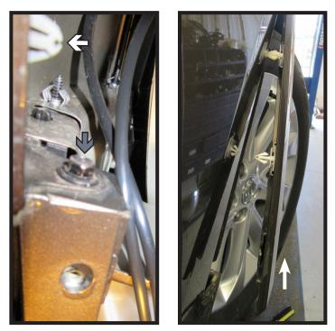
4. Pull back the wheel well liner. Using a 10MM socket remove the bolt (gray arrow). Then release the clips from the fender flare (left, white arrow). Pull straight up on the flare to release the bottom and then out away from the vehicle. Do this on both sides of the vehicle.
