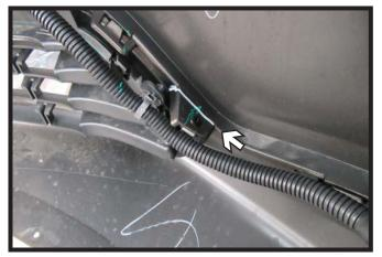
14. On the backside of the fascia, trim the lower tab back flush with the lip. Do this on both sides of the fascia.
