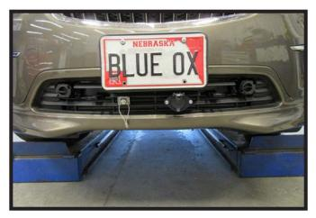
15. Hold the fascia as close to its original position, mark and trim the fascia around the convenience links and attachment tabs. Reinstall the fascia and fascia cover.
