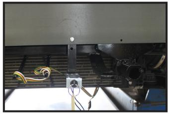
15. **Optional Breakaway:** Install the breakaway bracket to the existing hole in the bumper and the breakaway switch to the bracket with the supplied 1/4" hardware.
