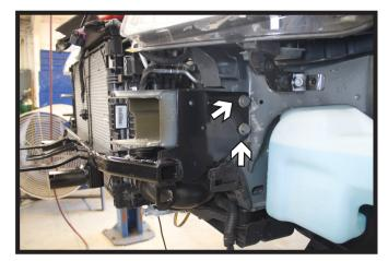
11. Position the baseplate onto the frame.
