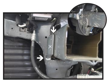
Using a reciprocating saw, trim flange off the side of the frame for baseplate clearance. Do this on both sides of the vehicle.
