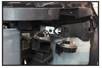
Using a 13MM socket, remove the screw from the horn bracket on the driver side and set the horn assembly aside.
