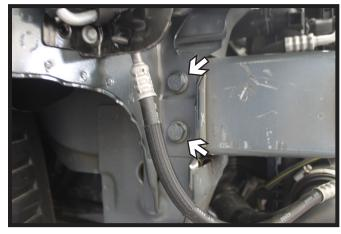
9. Using a 18MM socket, remove the four (4) bolts from the frame. There are two (2) on each side.
