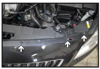
1. Using a T20 Torx, remove the six (6) screws from the top edge of the fascia. There are three (3) on each side.
