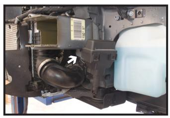
8. On the driver side, unsnap the fuse box from the post and set aside for baseplate installation.
