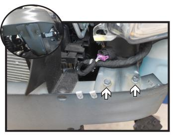
7. Using a 13MM socket and wrench, remove the four (4) bolts and nuts from the bumper. There are two (2) on each side. Set the bumper aside.
