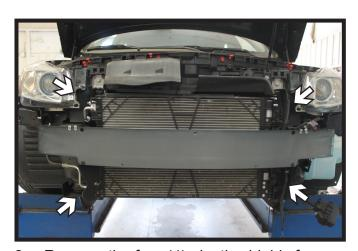
6. Remove the four (4) plastic shields from the vehicle by removing the push pins located on the bumper, top and bottom of the vehicle. These will not be reinstalled.
