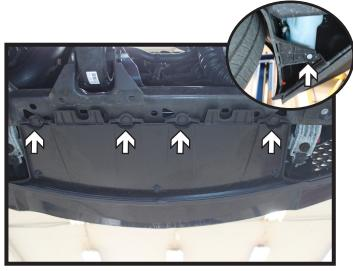
3. On the underside of the fascia, remove the four (4) push pins towards the center. Using a 8MM socket, remove the two (2) screws from the outer edges of the fascia. There is one (1) on each side (inset).
