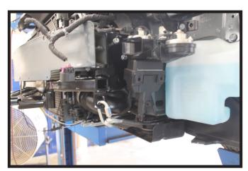
14. Reinstall the bumper, fuse box, horn assembly, intake tube and plastic supports.
