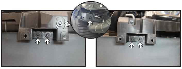
5. Using a 7MM socket, remove the five (5) screws from the plastic supports. There are three (3) on the passenger side (left) and two (2) on the driver side (right). Unclip the supports back towards the headlight and set them aside.
