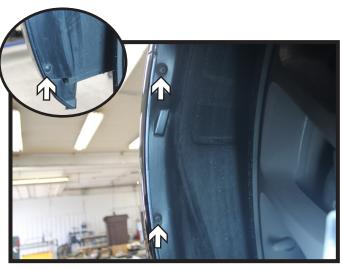
2. Using a T20 Torx, remove the two (2) upper screws from the edge of the wheel well. Then using a T15 Torx, remove the lower screw from the edge of the wheel well (inset). Do this on both sides of the vehicle.
