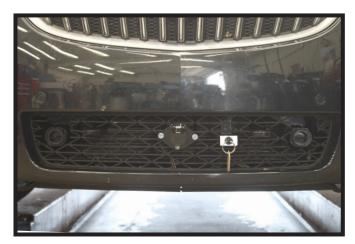
16. Hold the fascia as close to its original position, mark and trim the fascia around the convenience links and attachment tabs. Reinstall the fascia.
