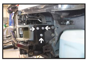
12. Using a 3/8" drill bit, drill the remaining holes thru the frame. Install 3/8"-16 x 1-1/2" bolts with lock washers into the holes and 3/8" nut plates on the inside of the frame. Do this on both sides of the vehicle. Fully tighten all hardware.
