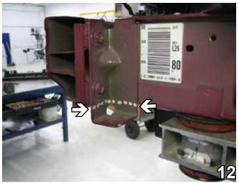
12. Using the reciprocating saw, mark and cut the bottom of the bumper bracket so that it is flush with the bottom of the frame rail. Do this to both sides of the vehicle.
