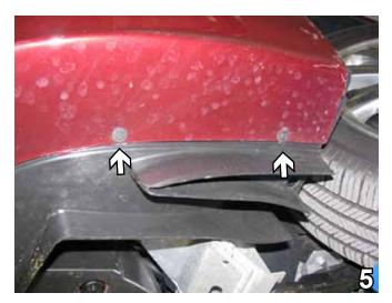
5. Using the 7mm socket, remove two metric bolts from underside of fascia, just forward of front tire. Do this to both sides of the vehicle. Set bolts aside to be reinstalled later.
