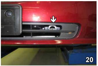
Align the fascia to its original position and, using the hack saw blade, trim necessary openings in the grille for the attachment tabs. Do this to both sides of the vehicle.
