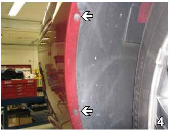
4. Using the 7mm socket, remove two metric bolts from just inside wheel well in front of the tire on the edge of the fascia. Do this to both sides of the vehicle. Set bolts aside to be reinstalled later.
