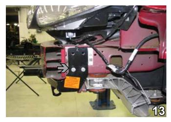
13. Align the baseplate with the webbing at the top of the frame rail and the contour on the back edge of the frame rail. Clamp in place with the vise grips. Using the baseplate as a template with the13/32" drill bit, drill the lower left hole (gray arrow). Be sure the baseplate is level with the frame. Drill the remaining three holes. Do this to both sides of the vehicle.
