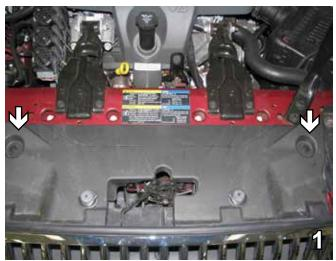
1. Remove two push pins from the top of the plastic cover. Set cover and push pins aside to be reinstalled later.
