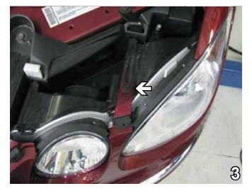
Remove the push pin from between the headlights. Do this to both sides of the vehicle. Set push pins aside to be reinstalled later.
