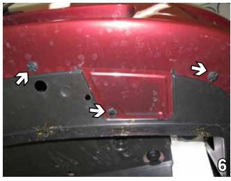
6. Remove three push pins from bottom corner of fascia. Do this to both sides of the vehicle. Set push pins aside to be reinstalled later.
