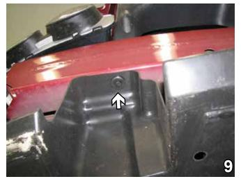
9. Remove two push pins from the belly pan extensions one on each side. Set push pins aside to be reinstalled later.
