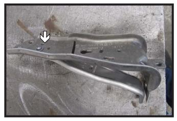
15. Using a T30 Torx, remove the bolt holding the secondary bracket to the primary bracket. Do this for both side brackets.
