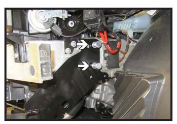
13. Slide the baseplate onto the vehicle, make sure it is level. Start the top two (2) 3/8" bolts. Do this on both sides of the vehicle.
