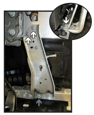
9. Using a T30 Torx, remove the three (3) bolts (white) holding the side bracket. Then using an 8MM socket remove the one (1) bolt (gray). Do this on both sides of the vehicle.
