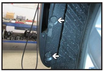
Using an 8MM socket remove the two (2) bolts from along the edge of the wheel well. Do this on both sides of the vehicle.
