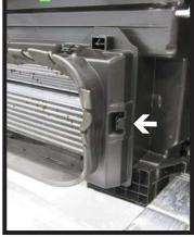
10. Remove the shroud surrounding the grill by releasing the ten (10) clips holding it in place. There are four (4) clips on the top, four (4) on the bottom, and one (1) on each end. Set aside to be reinstalled later.
