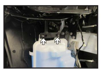
8. On the passenger side of the vehicle use a T30 Torx, remove the two (2) bolts at the top of the windshield washer reservoir. Unplug all lines and remove reservoir, set aside to be reinstalled later
