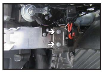
11. Using a 18MM socket remove the two (2) bolts from side of the bumper. Do this on both sides of the vehicle.
