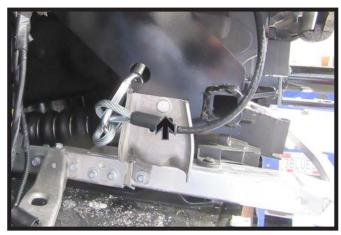
17. Reattach side bracket to frame by starting the bottom rear bolt (white) and the bottom front bolt (gray). Then using the hole from the baseplate as a guide drill a 3/8" hole (black) into the bracket and secure bracket to baseplate using 3/8" hardware. Do this on both sides of the vehicle.
