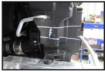
12. Measure 2" down from the top of the plastic piece and draw a line straight across. Then measure 2" down from the first line and draw a second line straight across. Trim the entire indicated area between the two (2) lines. Do this on both sides of the vehicle.
