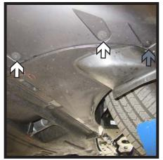
7. Remove the two (2) push pins (gray) from the under side of the fascia, one (1) on each side. Then using an 8MM socket remove the seven (7) bolts (white) from the under side of the fascia. Then remove the fascia and set aside to be reinstalled later.
