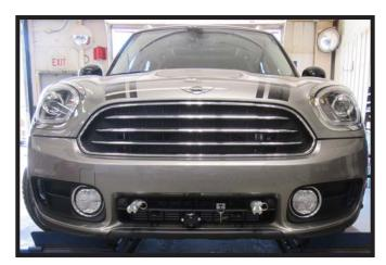
20. Hold the fascia as close to its original position, mark and trim the fascia around the convenience links and attachment tabs. Reinstall the fascia.
