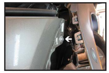
Using a T30 Torx, remove the bolt from under the fender. Do this on both sides of the vehicle.
