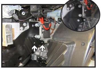
14. After starting the first two (2) bolts, use a 3/8" drill bit to drill out the bottom two (2) holes. Then insert the 3/8" hardware. Do this on both sides of the vehicle.
