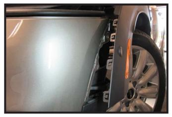
5. After releasing two (2) clips from the back side, pull outward on the fender to release the remaining four (4) clips. Do this on both sides of the vehicle.
