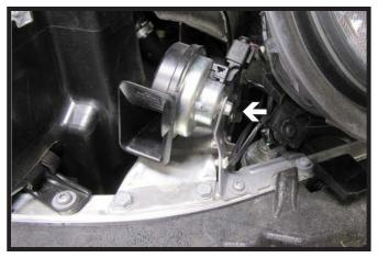
6. On the driver side, using a 10MM socket, remove the one (1) screw from the upper horn and set aside.
