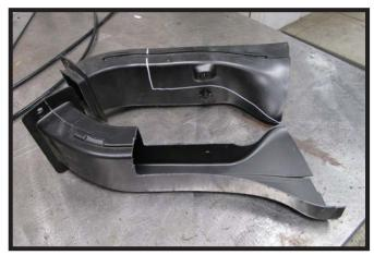
13. Using a reciprocating saw, trim both of the plastic air baffles as shown before reinstallation.
