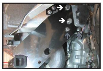
Install the baseplate to the vehicle using the existing frame holes with the provided 12MM hardware (white). Level and fully tighten all bolts.
