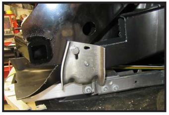
14. Using a reciprocating saw, trim the bumper support brackets as shown.
