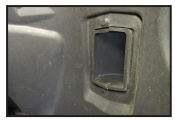
8. Remove the two (2) push pins from the plastic inside the wheel well, and remove the air baffle. Do this for both sides of the vehicle.
