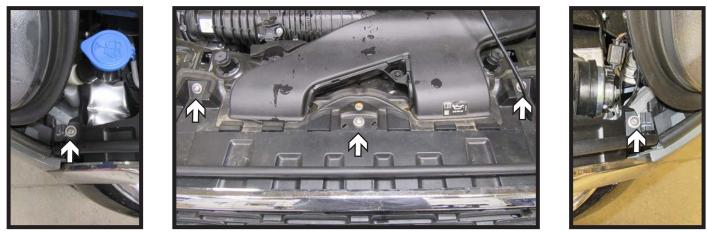
1. Using a T30 Torx, remove the five (5) screws from the top edge of the fascia.
