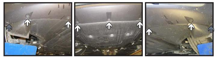
4. Using an 8MM socket, remove the seven (7) screws from the underside of the fascia (white). Remove the two (2) push pins from the edges of the underside (gray).
