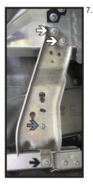
Using a T30 Torx, remove the two (2) screws from the top of the support bracket. Using a 8MM socket. remove the one (1) bolt from the bottom of the support bracket (black). Using a T25 Torx, remove the one (1) screw from the center of the support bracket (gray). Do this for both sides of the vehicle.
