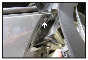
Pry the fender flare away from vehicle. Using a T30 Torx, remove the one (1) screw from behind the fender flare. Do this on both sides of the vehicle.
