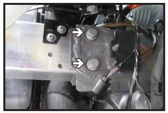
10. Using an 18MM socket, remove the two(2) bolts from the bumper horn. Do this for both sides of the vehicle.
