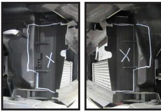
11. Using a reciprocating saw, trim the plastic shielding as shown on both sides of the vehicle for baseplate clearance.
