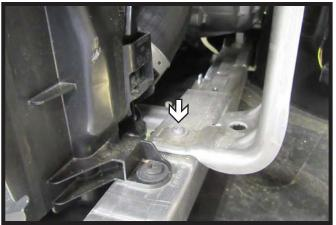
9. Using a T30 Torx, remove the one (1) screw from the metal brackets. Remove the bracket and set aside. Do this for both sides of the vehicle.
