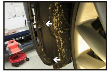
2. Using an 8MM socket, remove the two (2) screws from the outer edge of the wheel well. Do this on both sides of the vehicle.
