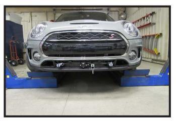
16. Hold the fascia as close to its original position, mark and trim the fascia around the convenience links and attachment tabs. Reinstall the windshield wiper fluid reservoir, fascia and fascia cover.
