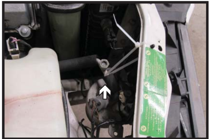
14. Using a zip tie, secure the hose to the car frame to ensure it remains out of the way during cutting.
