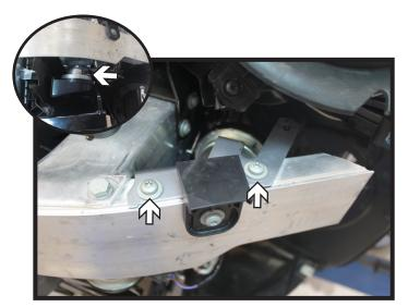
13. Reinstall the bracket to the vehicle. After the bracket is reinstalled reattach the upper horn to the bracket.
