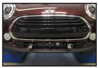
16. Hold the fascia as close to its original position, mark and trim the fascia around the convenience links and attachment tabs. Reinstall the washer reservoir and fascia
