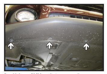
3. Using a 8MM socket, remove the seven (7) screws from the underside of the fascia.
