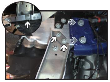
7. Using a T30 Torx, remove the two (2) screws from the top of the support bracket. Using a 8MM socket, remove the bolt from the bottom of the support bracket (inset). Set the bracket and 8MM bolt aside.
