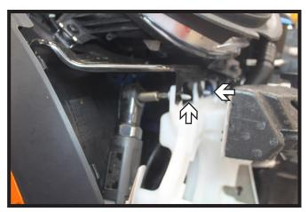
Using a T30 Torx, remove the two (2) screws from the washer reservoir. Disconnect/Plug all lines and set the reservoir aside.
