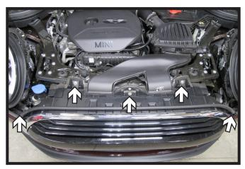
1. Using a T30 Torx, remove the five (5) screws from the top edge of the fascia.
