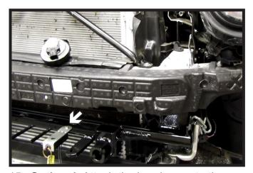
15. **Optional:** Attach the breakaway to the baseplate in the desired location with the supplied 1/4" hardware.
