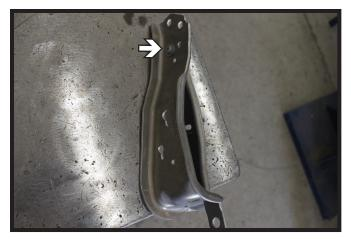
Remove the back strap from the support brackets by removing the T30 screw towards to top.
