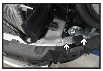
6. On the driver side, using a 10MM socket, remove screw from the upper horn and set aside (gray). Using a T30 Torx, remove the two (2) screws from the horn bracket (white). Disconnect all lines and set the horn assembly aside.
