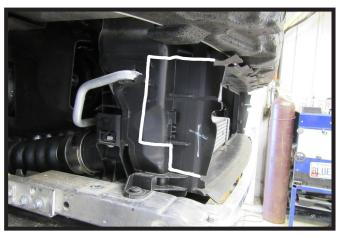
Trim the plastic shielding as shown on both sides of the vehicle for baseplate clearance.
