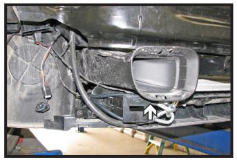
22. Reinstall the brake duct baffles on both sides of the vehicle.
