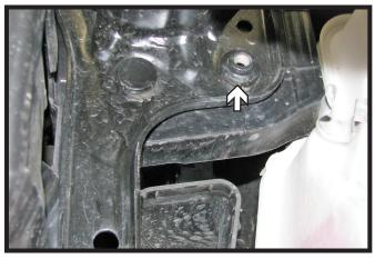
Using a 16MM socket, remove the bolt from the backside of the middle bumper bracket. Do this on both sides of the vehicle.
