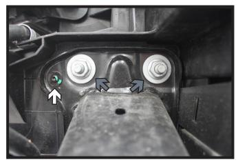
12. Using a T20 Torx, remove the screw from the top side of the bumper (white).
