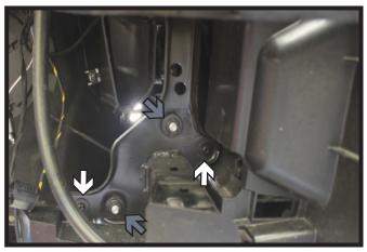
14. Using a T20 Torx, remove the two (2)screws from the bottom side of the bumper (white).
