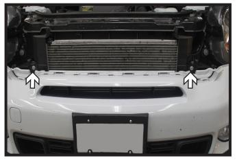
4. Using a T25 Torx, remove the two (2) screws from the top edge of the fascia.
