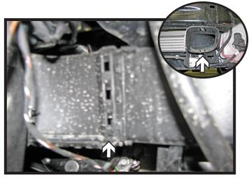
9. In front of the wheel well, using a flat screwdriver, disconnect the brake duct baffle and set aside. Do this on both sides of the vehicle.
