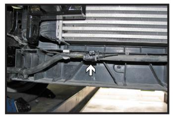
20. Reinstall the bumper/baseplate to the vehicle with the existing hardware. Reinstall the washer fluid line back into the clips. Then zip-tie the temperature sensor to the washer fluid line as shown.
