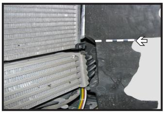
Trim the lower portion of the plastic shrouding off as shown for baseplate clearance. Do this on both sides of the vehicle.
