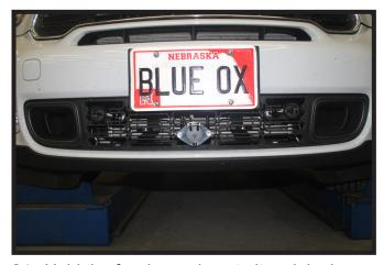
24. Hold the fascia as close to its original position, mark and trim the fascia around the convenience links and attachment tabs. Reinstall the fascia, grille and fascia cover.
