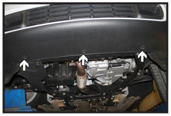
8. Remove the three (3) push pins from the underside of the fascia towards the middle of the vehicle.
