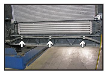
Unsnap the washer fluid line from the three (3) clips for easier bumper/baseplate installation.
