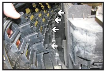
3. Using a flat screwdriver, push down on each of the four (4) clips going across the bottom of the grille to release it from the fascia. Do this on both sides of the vehicle. Set the grille aside.
