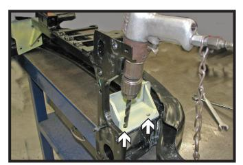
16. Using a 13/32" drill bit, drill the bottom two (2) holes in the baseplate thru the bumper. Install 3/8"-16 x 1-1/4" bolts with 3/8" lock washers into the holes and 3/8"-16 nut plates on the inside of the bumper, using the flat washers in between the bumper and baseplate as spacers. Do this on both sides of the bumper. Tighten all fasteners.
