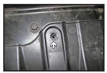
23. **Optional:** Attach the breakaway to the bracket with 1/4"-20 x 3/4" bolt and 1/4"-20 nut (left). Insert the breakaway switch into the grille opening in line with the center bolt hole on the driver side of the fascia cover. Reinstall the grille and the cover. Attach the breakaway bracket with an existing bolt inserted from the top of fascia cover that was removed in step 1 (right).
