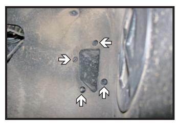
10. Using a 8MM, remove the four (4) screws from inside the wheel well that hold the on the brake duct. Set the duct aside, this will allow access to bumper bolts later on. Do this on both sides of the vehicle.
