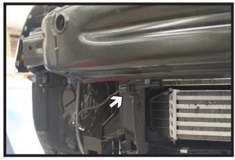
11. On the passenger side under the bumper, remove the temperature sensor from the plastic shrouding. The sensor will be relocated after baseplate installation.
