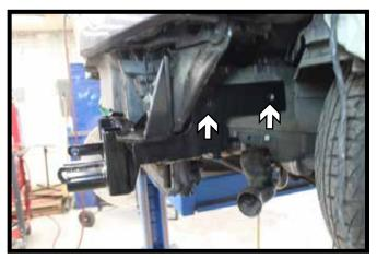
10. Using a 13/32" drill bit, drill the two (2) holes in the side of the baseplate thru the frame. Install 3/8"-16 x 1-1/2" bolts with 3/8" lock washers into the holes and 3/8"-16 nut plates on the inside of the frame. Do this on both sides of the vehicle. Fully tighten all fasteners.
