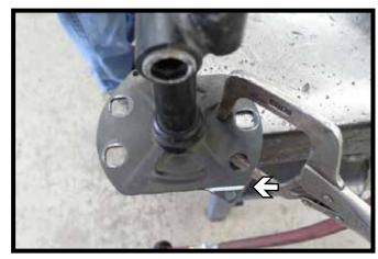
8. On the bumper support, trim off the lower tab. Do this on both supports.
