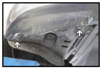
Using a 8MM socket, remove the four
