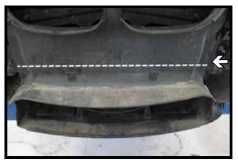
6. Trim the air dam off just below the bolt heads across to allow baseplate clearance.
