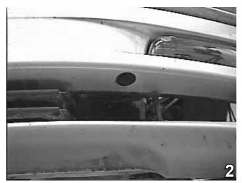
Remove the #12 Torx bolts from below the headlight. Do this on both sides of the vehicle. Set bolts aside to be reinstalled later. Unplug the running lights, and pull the fascia forward from the vehicle. Set the fascia carefully aside to be reinstalled later.
