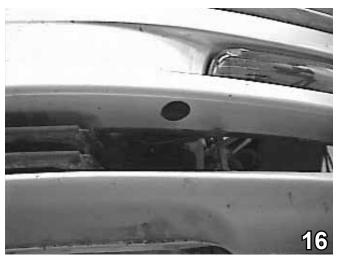
16. The two outside grille pieces need to be removed (snapped into place) to allow the attachment tabs to be used. Keep the pieces for when the cat is not being towed.
