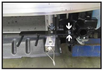
11. Install the electrical mounting bracket to either side convenience link using two (2) 5/16" bolts (white) with nylon lock nuts.
