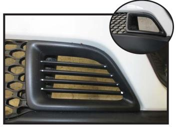
13. Remove the horizontal slats from the corner of the fascia as shown. Do this on both sides of the vehicle.
