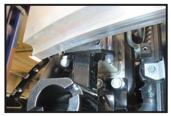
10. Attach flat piece above the bumper to the baseplate using two (2) 3/8" x 4-1/2" bolts and nylon lock nuts. Do this on both sides of the baseplate.
