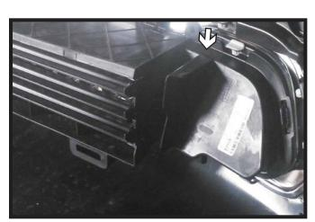
12b. Shutter Models: The plastic surrounding the outer grille areas must be trimmed to expose the grill behind. Follow the protrusion straight down leaving the areas next to the screws intact. Do this on both sides of the fascia.
