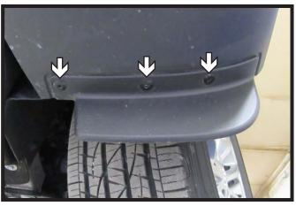
3. Using a 1/4" drill bit, drill out and remove the three (3) pop rivets underneath the vehicle in front of the tire. Do this on both sides of the vehicle.
