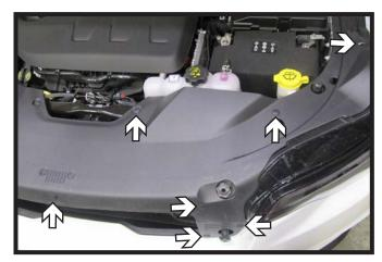
1. Remove the thirteen (13) push pins from the top edge of the fascia cover. There are six (6) on each side and one (1) in the center. Remove fascia cover and set aside to be reinstalled later.
