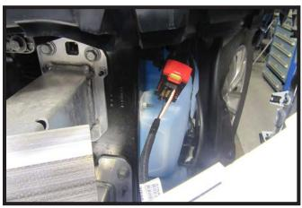
6. As the fascia is removed unhook the plug on the driver side by pulling out the yellow piece and up on the red part to unhook. Remove fascia and set aside to be reinstalled later.
