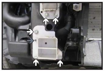
7. Using a 15MM socket, remove the three (3) bolts from the frame extension and two (2) bolts from the bottom side of the bumper (white). Using a 10MM socket, remove the nut (gray) from the fascia extension. Do this on both sides of the vehicle. The frame extension will not be reinstalled.
