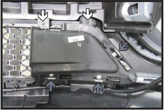
12a. Non Shutter Models: Using a 7MM socket, remove the two (2) bolts (white) from the air dam on the back side of the fascia. Unclip the three (3) clips (gray) by pushing down on the inside of the clip. Remove the air dam. Do this on both sides of the vehicle.
