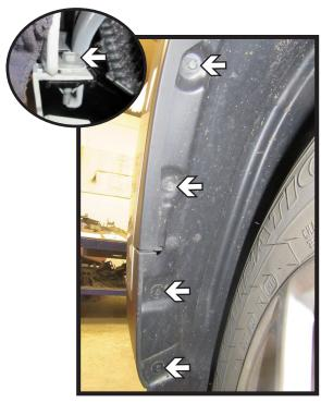
Using an 8MM socket, remove the four (4) bolts from the edge of the wheel well. Pull back the wheel well cover, using a 10MM socket, remove the bolt behind the trim (inset). Do this on both sides of the vehicle.
