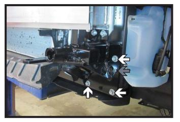
Insert the three (3) existing 10MM bolts with 3/8" flat washer and lock washer (white) and one (1) nut (gray). Tighten all hardware fully. Do this on both sides of the vehicle.
