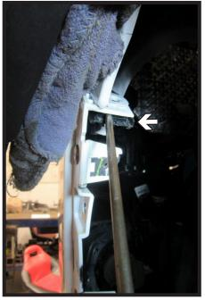
Unclip the wheel well trim from the backside. Then insert a flat head screw driver between black and white pieces as shown and pull the fascia outward to remove. Do this on both sides of thee vehicle.
