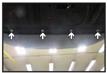
4. Using a 10MM socket, remove the four (4) bolts on the underside of the vehicle.
