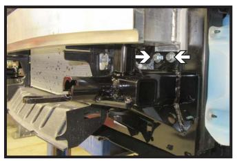
8. Slide the baseplate into place and start the two (2) 10MM bolts with 3/8" flat washers and lock washers on the bottom of the bumper. Do this on both sides of the vehicle.
