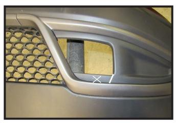
Trim the indicated area on the fascia to allow room for the baseplate. Do this on both sides of the vehicle.
