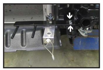
Install the electrical mounting bracket to the driver side convenience link using two (2) 5/16" bolts (white) with nylon lock nuts.
