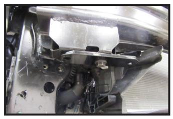
8. Loosely bolt the bumper attachment plate to the underside of the bumper with the existing 10MM hardware. Make sure the bumper plate is at the correct angle by holding up the baseplate and checking that the holes line up. Only install loctite onto the center bolt (white) and fully tighten. Once the center bolt is tightened, remove the outer bolt (gray) until the baseplate is installed. Do this on both sides of the vehicle.
