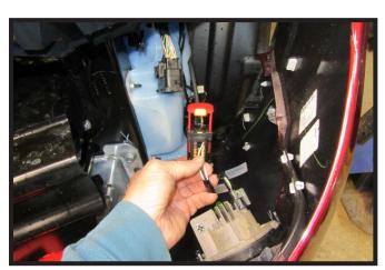
4. Lift the corner of the fascia up towards the fender and out to release. Continue along under the headlights unsnapping the fascia from the vehicle. As the fascia is removed unhook the plug on the driver side by pulling out the yellow piece and up on the red part to unhook. Remove fascia and set aside to be reinstalled later.
