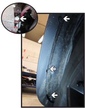
Using an 8MM socket, remove the three
