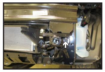
10. Reinstall the outer bumper attachment plate bolt (white). Start the 1/2" hardware on the inside edge of the plate (gray). Fully tighten all hardware. Do this on both sides of the vehicle.
