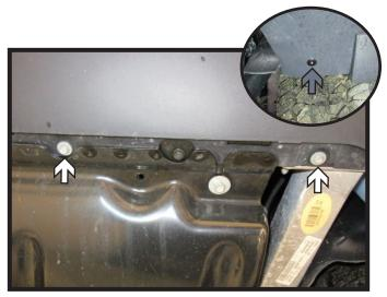
Remove the one (1) rivet (gray) from the underside corner of the fascia (inset).
