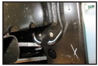
7. Using a reciprocating saw, trim the lower lip off the bottom of the bumper as shown so that it is flush with the face of for baseplate clearance. Do this on both sides of the vehicle.
