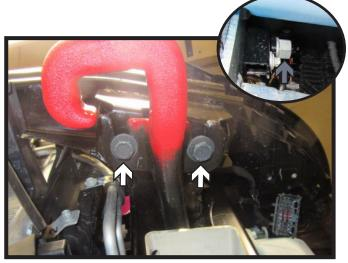
5. Using a 16MM socket, remove the two (2) bolts (white) from the underside of the tow hook. Using a 30MM socket, remove the nut (gray) from the backside of the tow hook and remove from the vehicle (inset). Do this on both sides of the vehicle.
