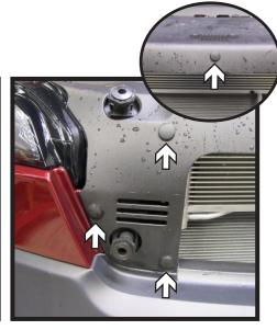
1. Remove the thirteen (13) push pins from the top edge of the fascia cover. There are six (6) on each side and one (1) in the center. Remove fascia cover and set aside to be reinstalled later.
