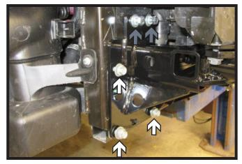
9. Install the baseplate to the vehicle using the three (3) existing extension bolts (white). Install 10MM bolts with 3/8" flat washers and 10MM lock washers into the lower bumper bolts (gray). Fully tighten all fasteners. Do this on both sides of the vehicle.
