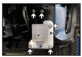
6. Using a 15MM socket, remove the three (3) bolts from the frame extension and two (2) bolts from the bottom side of the bumper (white). Using a 10MM socket, remove the nut (gray) from the fascia extension. Do this on both sides of the vehicle. The frame extension will not be reinstalled.
