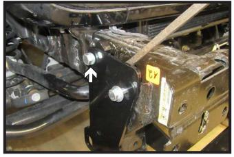
9. Loosen the top front bolt. Then insert spacer plate between the frame and the baseplate. Insert 1/2" bolt into back hole with lock washer and whiz nut. Turn the spacer plate so that it is flush with the baseplate and tighten bolt. Do this on both sides of the vehicle.
