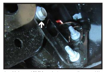
4. Using a 10MM socket remove the one (1) bolt on the outside of the frame holding the bracket after removing the bumper. Do this on both sides of the vehicle.
