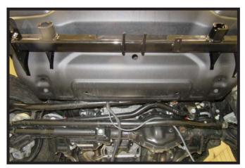
14. Hold the belly pan in place and trim as shown to allow room for the baseplate and electrical.
