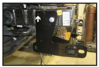
8. Using a 1/2" drill bit, drill out the top back hole on the outside of the frame using the baseplate as a template. Do this on both sides of the vehicle.
