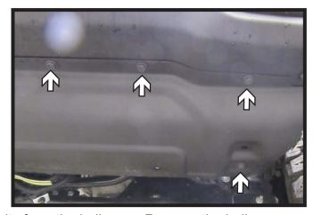
1. Using a 13MM socket remove the seven (7) bolts from the belly pan. Remove the belly pan and set aside to be reinstalled later.
