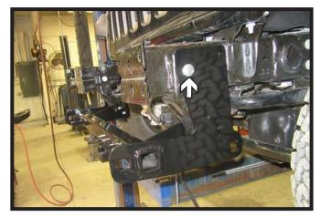
7. Slide the baseplate onto the vehicle. Start the front 10MM bolt with flat washer and lock washer. Snug bolt up tight so remaining holes line up but do not use Loctite® Red at this time. Do this on both sides of the vehicle.
