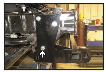
11. Install the 1/2" bolt with lock washer and whiz nut into the bottom hole on the outside of the frame. If the hole does not completely line up ream out hole with drill bit. Do this on both sides of the vehicle.
