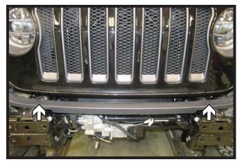
Remove the two (2) push pins holding the plastic piece to the frame. Set aside to be reinstalled later.
