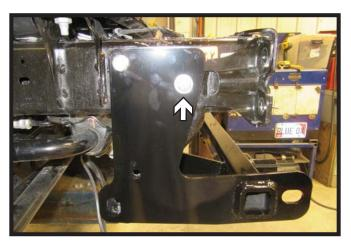
10. Remove the top front bolt and insert frame bracket between the frame and the baseplate. Make sure the bracket is flush with the front of the frame. Reinstall bolt and hardware. Do this on both sides of the vehicle.
