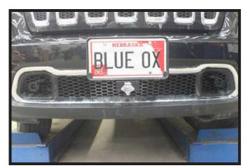
13. Hold the fascia as close to its original position, mark and trim the fascia around the convenience links and attachment tabs. Reinstall the fascia and fascia cover.
