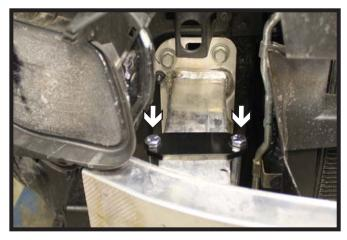
Install the support plate and bolts on top
