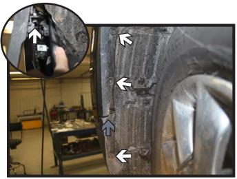
3. Using a 8MM socket, remove the three (3) screws from the edge of the wheel well. Using a 7MM socket, remove the one (1) screw at the fascia/trim joint (gray). Using a 10MM socket, remove the screw behind the trim (inset). Do this on both sides of the vehicle.
