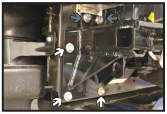
7. Install the baseplate to the vehicle using the three (3) existing extension bolts (white). Install 10MM-1.25 x 40MM bolts with 3/8" flat washers and 10MM lock washers into the lower bumper bolts (gray). Snug all fasteners, do not fully tighten. Do this on both sides of the vehicle.
