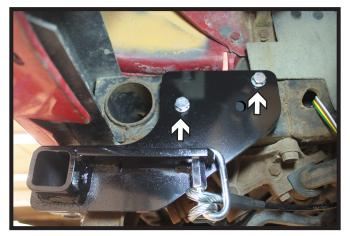
Using a 16MM socket, remove the two
