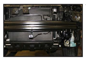
13. **Optional:** If installing a breakaway, screw the breakaway bracket to the bumper at the desired location with the #10-16 x 1" self drilling screw. Attach the breakaway to the bracket with a 1/4"-20 x 3/4" bolt and 1/4"-20 lock nut.
