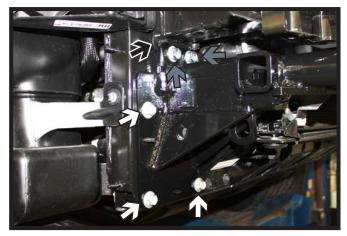
Install the baseplate to the vehicle using the three (3) existing extension bolts (white). Install 10MM-1.25 x 40MM bolts with 3/8" flat washers and 10MM lock washers into the lower bumper bolts (gray). Fully tighten all fasteners. Do this on both sides of the vehicle.
