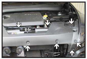
1. Remove the twelve (12) push pins from the top edge of the fascia cover and set aside.
