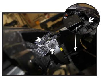
Using a 10MM socket, remove the three
