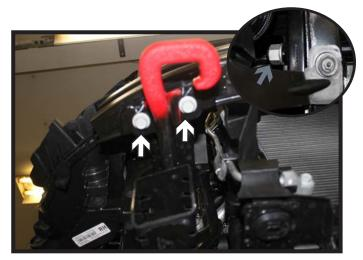
Using a 16MM socket, remove the two (2) bolts from the underside of the tow hook (white). Using a 30MM socket, remove the nut from the backside of the tow hook and remove from the vehicle (inset). Do this on both sides of the vehicle.
