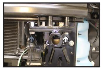
Reinstall the outer bumper attachment plate bolt (white). Install the 1/2" hardware on the inside edge of the plate (gray). Fully tighten all fasteners. Do this on both sides of the vehicle.
