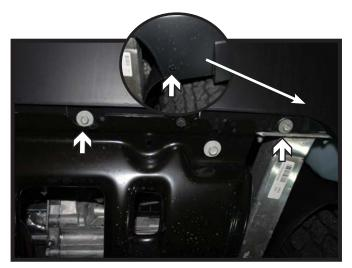
Remove the two (2) rivets from the underside corners of the fascia (inset). There is one (1) on each side. Using a 10MM socket, remove the four (4) screws from the middle portion of the fascia. There are two (2) on each side.
