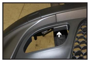
Trim the fascia opening as shown for clearance around the baseplate. Do this on both sides of the fascia.
