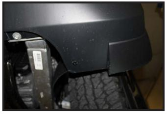
16. Install the new plastic rivets into the underside of the fascia, where the factory rivets were removed.
