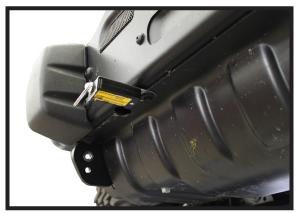
4. Align the hole of the breakaway switch bracket and use the fasteners provided.
