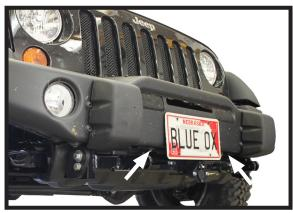
If installing a breakaway switch, use a 13MM socket to remove one (1) of the existing bolts on either side of the bumper.
