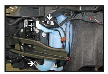
Using a 8MM socket, remove the two
