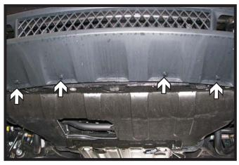
1. On the bottom side of the fascia, remove the four (4) push pins.
