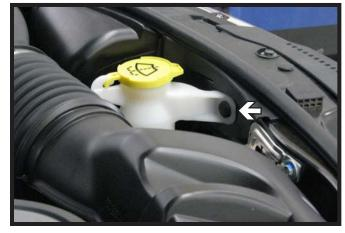
In the engine compartment, remove the push pin from the washer reservoir filler tube neck.
