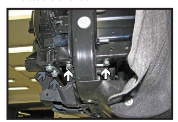
7. **Models equipped with tow hooks:** Slide the baseplate into position on the frame. Install two (2) 10MM-1.5 x 80MM bolts with 10MM lock washers into the bottom holes (white). Install a 3/4"Ø x 1-23/32" spacer tube with a 10MM-1.5 x 100MM bolt, 10MM lock and flat washer thru the spacer into the frame into both the front holes (gray). Tighten all hardware. Do this on both sides of the vehicle.
