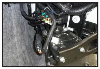
12. Loosely reinstall the compressor, checking for clearance around the baseplate. If needed shim the compressor away from the baseplate with 5/16" washers. This with keep the compressor from vibrating against the baseplate.
