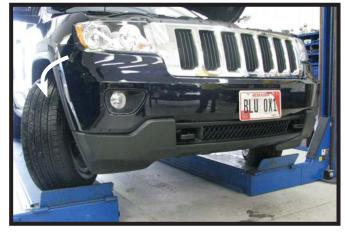
4. Pull the top corners of the fascia out releasing the clips behind. Continue working inward towards the grille releasing the clips under the headlights and grille. Set the fascia aside.
