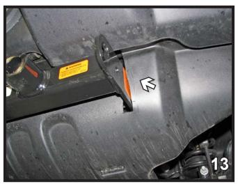
13. Hold the belly pan up to its original position, mark and trim a slot for baseplate endplate to come through with the utility knife. Do this to both sides of the vehicle. Slide the belly pan between baseplate crosstube and lower frame suspension. Allow endplate to come through slot and reinstall the belly pan to its original location.
