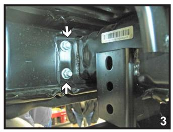
3. Disconnect the foglights from back side of bumper. Using a 18mm socket, remove the two (2) bolts on outside edge of frame. Do this on both sides of the vehicle.
