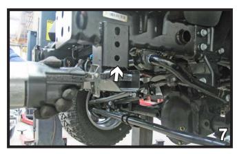
7. On the 2007-09 models: Align the baseplate's lower hole with the existing lower hole in the frame, insure baseplate is level with frame and clamp in place with the vice grips. Do this to both sides of the vehicle.
