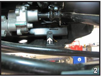
2. Using a Phillips screwdriver, remove the two (2) push pins from tabs on the backside of the belly pan. Set the belly pan aside.
