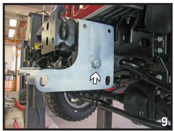
9. Insert the 5/8"-11 whiz nut into the frame end and align with the lower hole on the 2007-09s and the middle hole on the 2010s and newer. Install the 5/8"-11 x 1-1/2" hex bolt and 5/8" lock washer and tighten to whiz nut. Do this on both sides of the vehicle.
