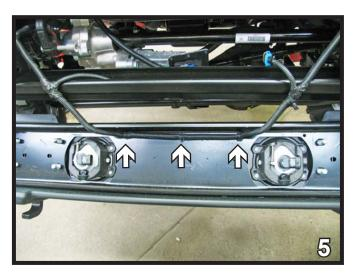
5. Pull the bumper forward and disconnect clips from the wiring loom running along the backside of the bumper. Set the bumper aside.
