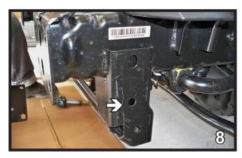
8. On the 2010 models and newer: Align the baseplate's lower hole with the existing middle hole in the frame, insure baseplate is level with frame and clamp in place with the vice grips. Do this to both sides of the vehicle.
