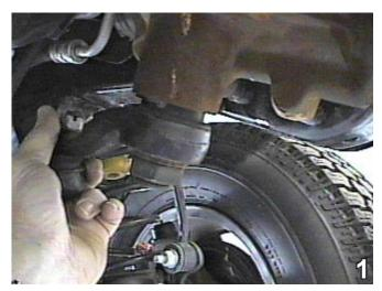
1. Remove three (3) metric bolts with the 16MM socket while having someone hold the gear box and the idler arm. Set metric bolts aside to be reinstalled later. Do this to both sides of the vehicle.
