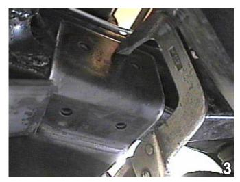
Clamp the baseplate on the passenger's side with the large vise grips. Using the baseplate as a template, drill four (4) holes with the 13/32" drill bit.
