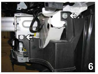
6. On the driver's side, remove the air baffle. Use a 10MM socket to remove the two metric bolts
