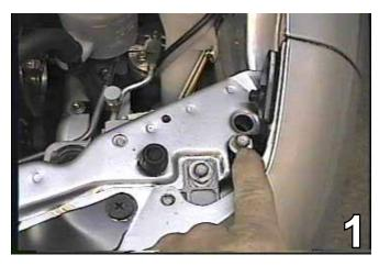
With the 10MM socket remove metric bolt on the top edge of the fascia, just above the headlight assemblies. Do this to both sides of the vehicle.
