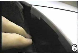
Pull black plastic back and remove one Phillips screw from inside fender that meets the fascia's outside corner. Do this to both sides of the vehicle. Disconnect the fog lights, pull fascia forward, and set it carefully aside to be reinstalled later.
