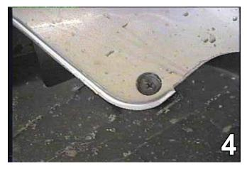
4. There is one Phillips screw to remove just outside of previous bolts on underside of the fascia. Do this to both sides of the vehicle.
