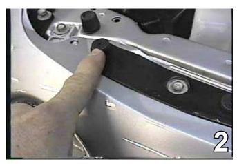
Remove the nine Phillips head bolts from the top of the fascia and set black support plate aside to be reinstalled later.
