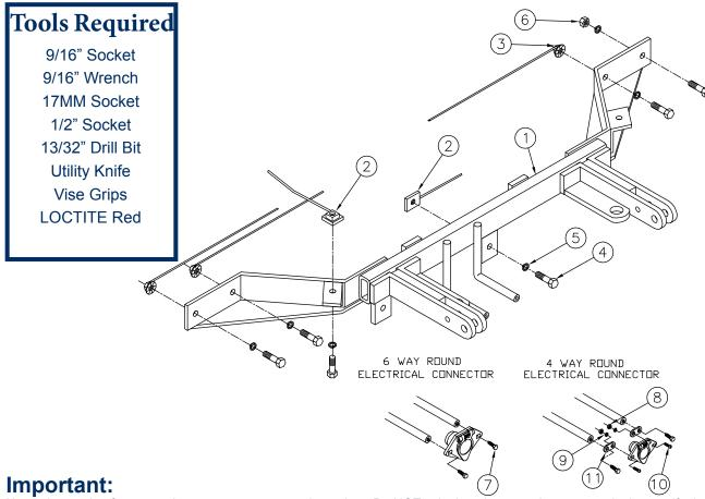
Use only genuine factory replacement parts on your baseplate. Do NOT substitute homemade or non-typical parts. If a bolt is lost or in need of replacement, for your safety and the preservation of your baseplate, be sure to use a replacement bolt of the same grade (In most cases it will be Grade 5, please reference the parts list above). Replacement parts may be ordered through your nearest Blue Ox® Dealer or Distributor, or call our 24/7 Customer Care Team at (402)385-3051.
