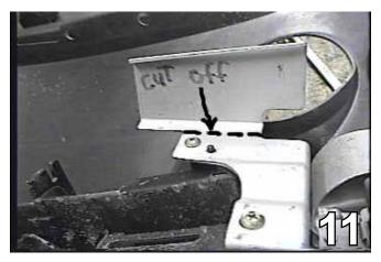
11. Cut off the metal supports on the inside of the fascia. **NOTE:** Cut at location of black line marked on the fascia, as indicated by the dotted line in the photo above.
